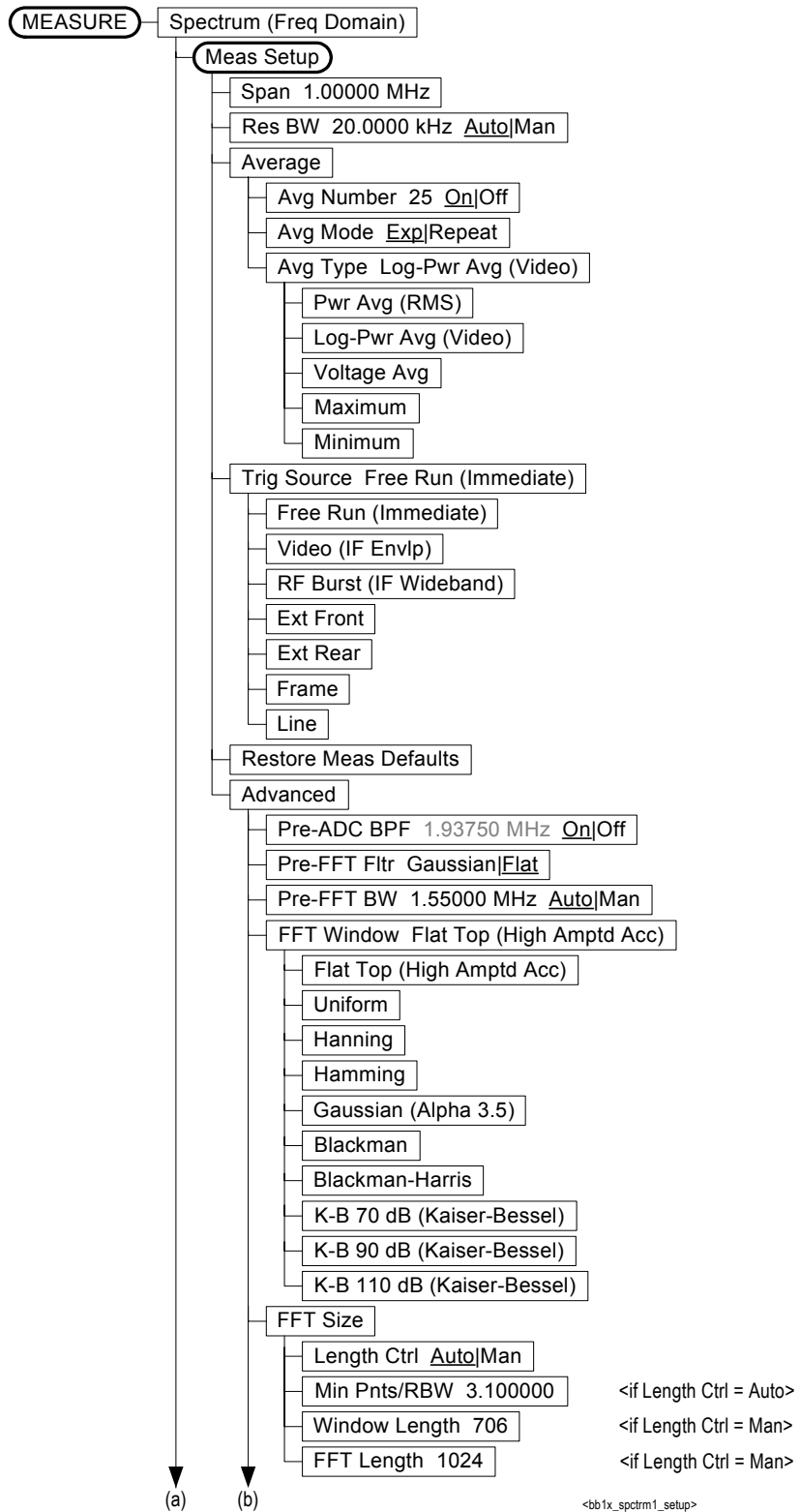
Figure 6-29 Spectrum (Freq Domain) Measurement Key Flow (1 of 4)
