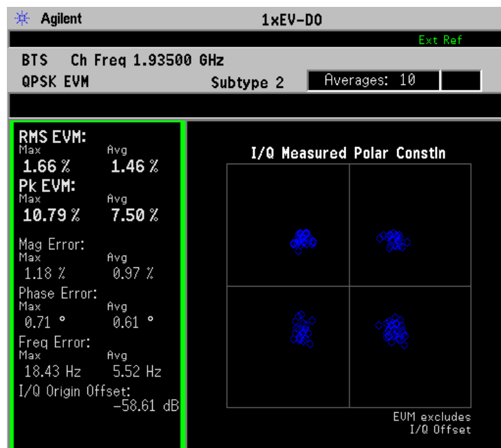
Figure 3-25 QPSK EVM Measurement - I/Q Polar Constellation View
