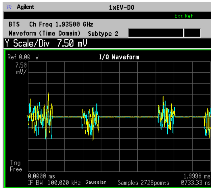
Figure 2-105 Waveform Measurement - I/Q Waveform View
