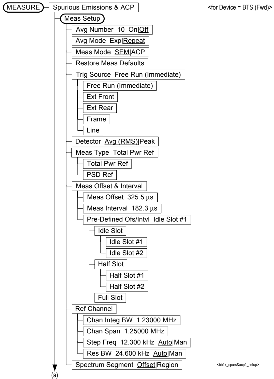
Figure 6-33 Spurious Emissions & ACP Measurement Key Flow (1 of 3)
